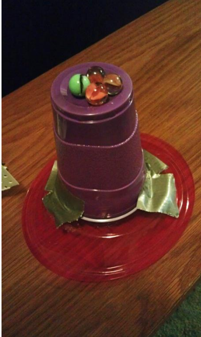
Example of a solar tracker utilizing ball bearings (marbles between plastic cups) and a four-bar linkage. The solar panel is attached to the long vertical member.
