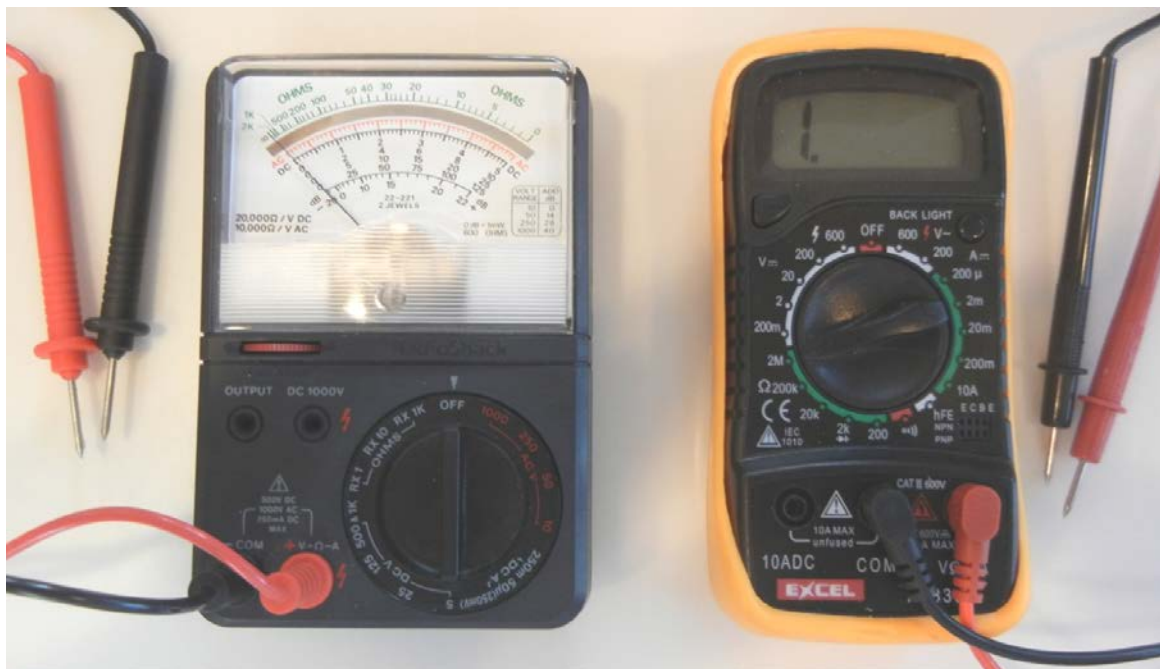
Figure 6: Analog (left) and digital (right) Ohmmeters. The red (positive) and black (negative) test leads are connected to the meters for DC voltage or resistance. On the analog meter (dial scale, numbers in green, measures resistance), the resistance settings are Rx 1 (measures resistance in Ohms directly), Rx 10 (multiply the resistance reading by 10 for actual resistance), and Rx 1K (multiply the resistance reading by 1000 for actual resistance). On the digital meter, the resistance settings are 2K (measures resistance in Ohms directly for 0-2000 Ohms range), 20K (multiply the resistance reading by 1,000 for actual resistance), 200K (multiply the resistance reading by 1,000 for actual resistance), and 2M (multiply the resistance reading by 1,000,000 for actual resistance). Always begin by using the highest setting (Rx 1K for the analog meter and 2M for the digital meter) and work your way to the lower settings until the dial can be easily read on the analog meter or until an appropriate digital number appears on the digital meter.
